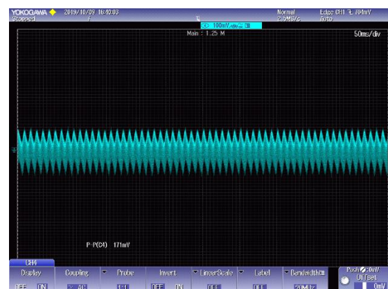
(b) 230 V (measured value=171 mV)
