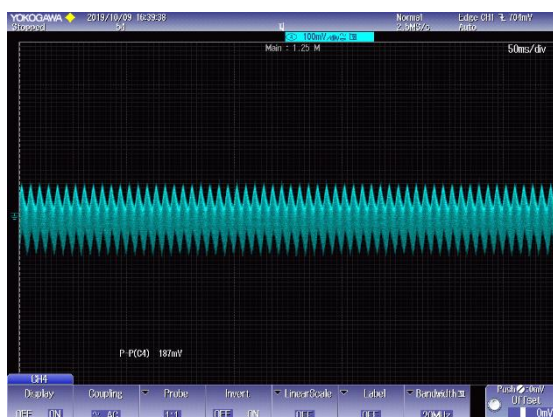
(a) 115 V (measured value=187 mV)
